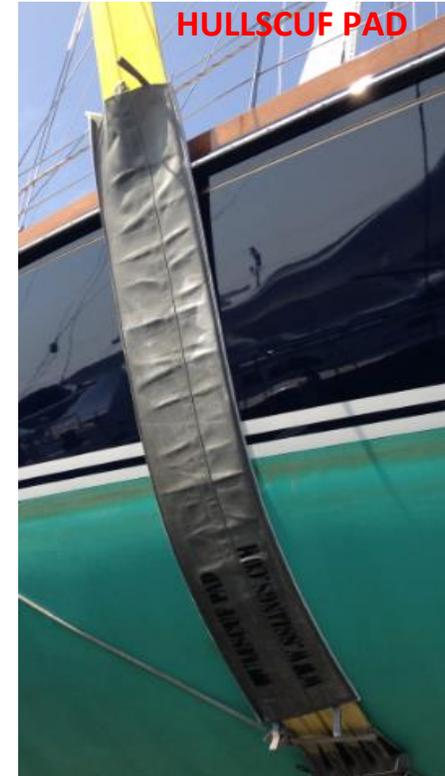
The **HULLSCUF PAD**, is a durable lightweight protective sleeve designed to slide over the sling. When in use, the **HULLSCUF PAD** helps reduce sling friction against the boat and minimizes hull marring. The **HULLSCUF PAD** is reusable after each launch and haul with a power wash. Keep your yard crew busy on important tasks and your customers satisfied after their fresh spring paint!
